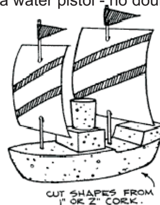
CORK SHIP. Carve hull and superstructure from one- or two-inch-thick pieces of scrap cork. Nail, pin, or glue on other parts and attach dowel masts and sails.
