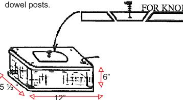
Surface apply a 6" strip of screen mesh by stapling to the top and bottom edges.
